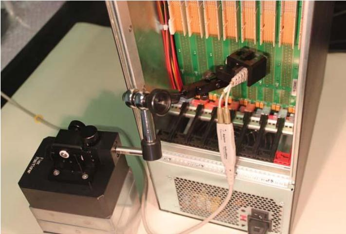
Flex Positioner for the vertical probing of a backplane
